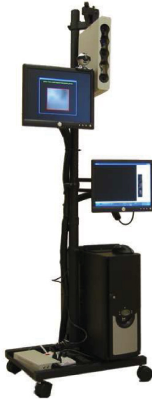
Fig. 10.10. Prototype system using a 3dMD TM optical scanner with a one-pod configuration
