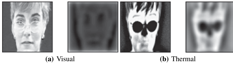
Fig. 6.5. Preprocessing : the effects of the optimal band-pass filters on registered and cropped faces in (a) visual and (b) thermal spectra
