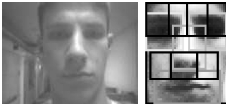
Fig. 9.1. A sample image and its face detection result with the face component regions superimposed
